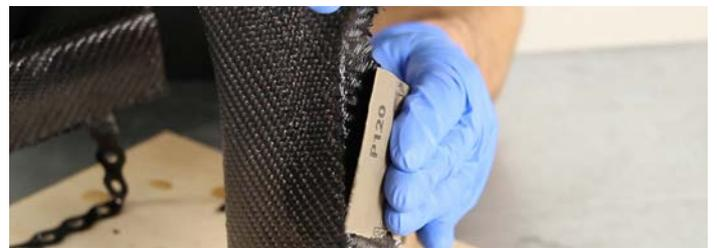
Once the 1st coat of resin has cured to a hard, sand-able finish, use a piece of 120 grit abrasive paper to remove any nibs (often caused by loose fibres at the edge of join-lines standing up), drips or other high spots.
