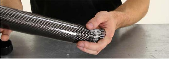
Carbon fibre fabric is very delicate. Even the process of removing the carbon fibre from the tube or roll can be enough to distort the fabric.
