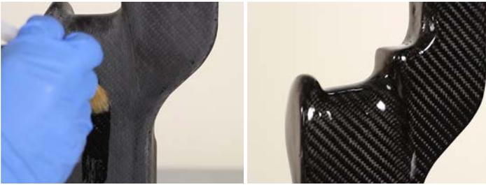
The final layer of resin only needs to be applied very thinly, almost like applying a varnish or lacquer to the part. The smooth surface underneath should make it possible to achieve a smooth, level gloss finish which looks good even before it is flatted and polished.
