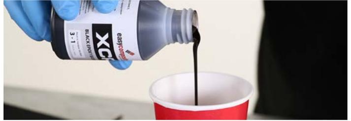
Mix a quantity of basecoat suitable for the size of the part that you are going to skin. To help you to work out the correct amount of basecoat, you'll need about 330g of basecoat (and hardener combined) to cover 1sqm of surface - this means that if you are using the whole of the 0.3sqm of carbon fabric included in the small skinning kit you would want to mix up around 100g of basecoat; if you used half this much fabric then you would only need 50g of mixed basecoat.
