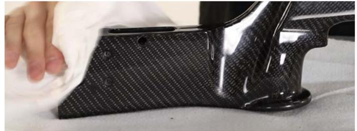
The NW1 compound can be used by hand or with a polishing pad and power polisher. Where available, a power polisher is likely to be much quicker than hand polishing.
