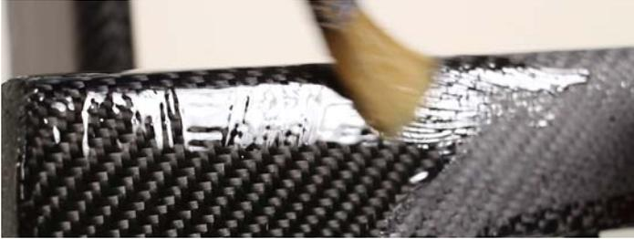
You must NOT allow the previous layer of resin to cure past the 'tack' stage before applying the next layer of resin. If you do, the new layer of resin will not be able to bond properly to the previous layer and could delaminate. You will also find that the new layer of resin will visibly 'fish-eye' away from the previous layer if it is no longer at the tack stage (see recovery method below).
