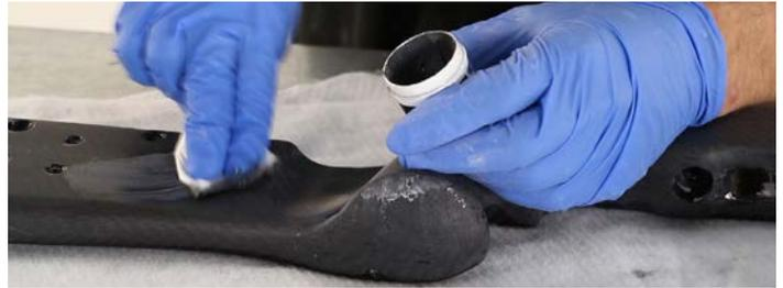
The NW1 Black Super Cutting Compound included with the Skinning Starter Kit and also available separately from Easy Composites should be used to polish the skinned part from a smooth but satin-finish 1200 grit finish up to a full gloss.
