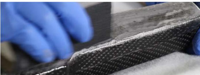
Once the clear layers of resin have cured to a fully hard finish there will now be enough thickness of resin to allow the surface to be properly flattened.
