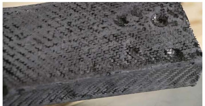
Next you'll need to key the whole surface of the part with more 120 grit paper so that the next layer of resin can bond to it. Whilst you can do some light 'flattening' at this stage (to remove high or low spots in the resin) be careful not to break through to the carbon fibre. If you see the sanding dust turn black then you should stop right away.
