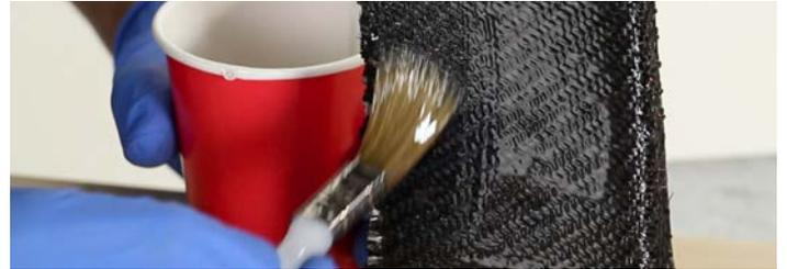
Apply an even coat over the whole surface of the part, making sure you fully wet-out the dry carbon fibre. You are never aiming to achieve a thick coat of resin with any single application; instead, thickness is built up using a number of thin layers.
