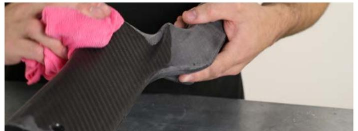
Before applying the final coat of clear resin it is very important to remove all sanding dust from the surface of the part because any dust that remains on the surface when the final coat of resin is added can contaminate the resin and will be visible in the final finish. This can be achieved using a tack-rag, microfibre cloth or by washing the part in mildly soapy water.
