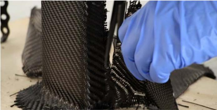
For complex parts you may need to consider completing the surface in multiple sections. With skill, join lines like this can be achieved very discreetly, especially when positioned on corners where they can be almost impossible to see. If you do need to achieve neat join-lines on your part then an epoxy compatible spray adhesive such as Easy Composites' FusionFix™ is required.
