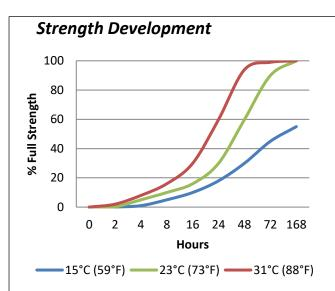
Graph shows typical strength development of bonded components. An increase of  $8^{\circ}$ C ( $46^{\circ}$ F) in temperature will halve the cure time. Lower temperatures will result in a slower cure time.
