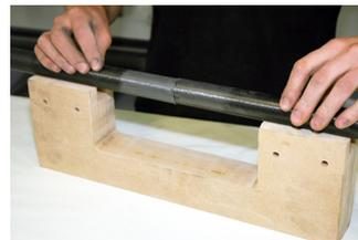
If repairing a pole that has been broken in two, align and support the two halves of the pole either side of where the repair will be made.
