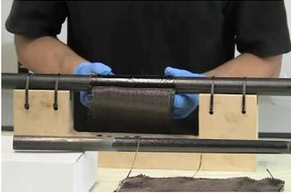
Taking the piece of cut carbon fibre fabric, align the fabric along the pole and press the leading edge of it onto the tacking resin.
