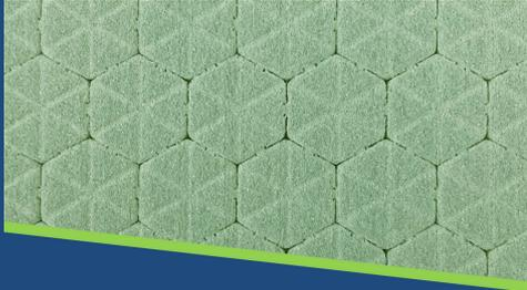
The 3D|CORE™ PET GR foam core is a green foam made from 100% recycled material. The core is a closed-cell, thermoplastic and recyclable rigid foam with excellent technical properties. It is suitable for the construction of high-strength lightweight components. The integrated honeycomb structure provides more flexibility and is easy to handle.
